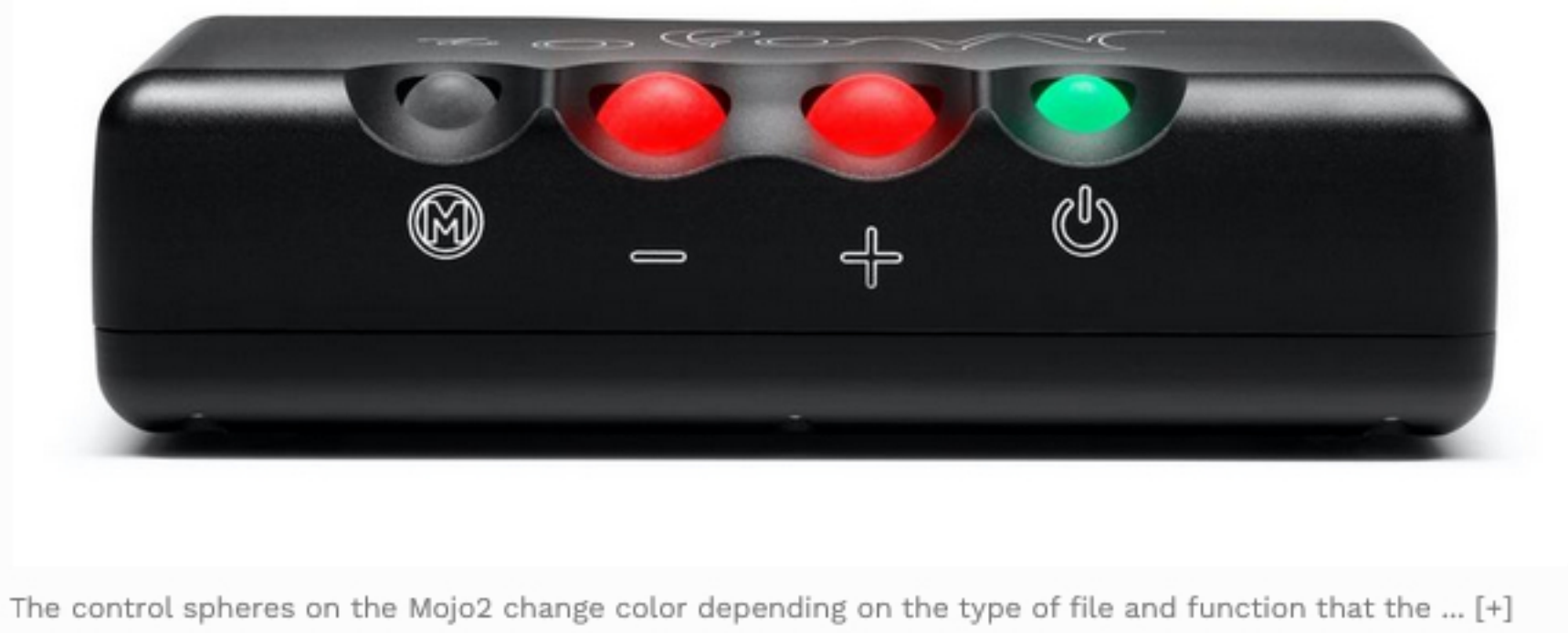
The control spheres on the Mojo2 change color depending on the type of file and function that the ... [+] CHORD ELECTRONICS
