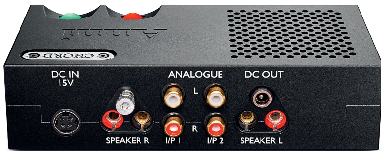
ABOVE: Two RCA line inputs are joined by inset 4mm banana plug (speaker) sockets and an earth/grounding post. The 15V DC PSU input also feeds a 12V DC output to power the Huei phono stage [see picture, below]
